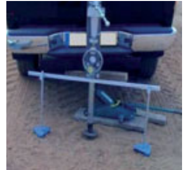
CBR Testing being carried out on site
